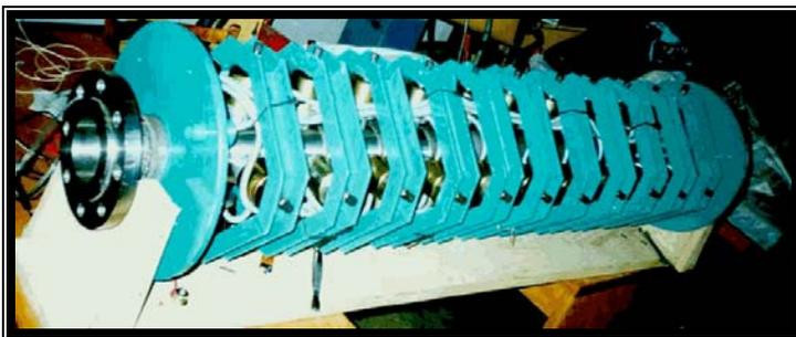
Ultrasound cavitation processor:  $d_y=100$  mm, power 2.0 kW, Capacity- 5500 gallons per hour
